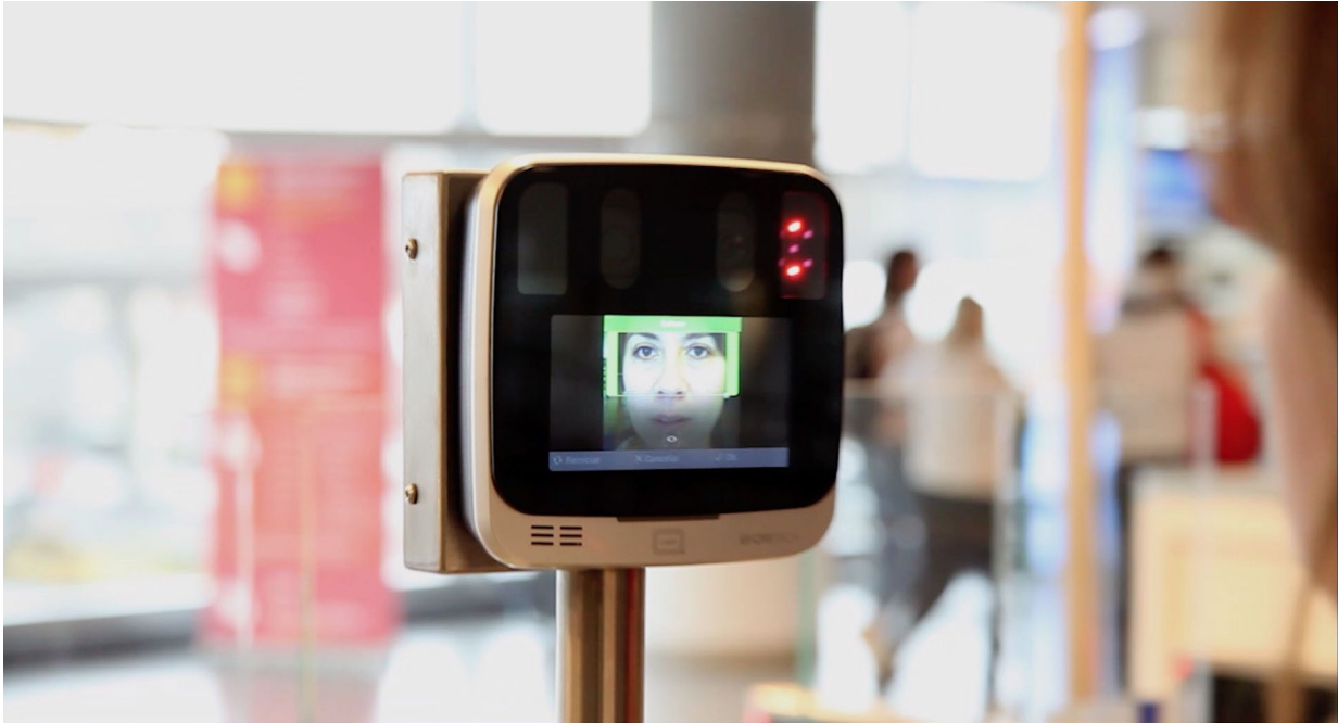
Iris recognition device used in the migratory process with the BioMig system.
